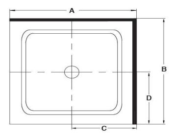
Minimalist low threshold 3" height Centre Drain Side & Back Wall Integral Flange
